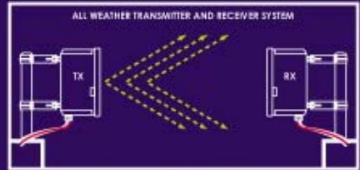
Mounting transmitter and receiver on the edge of a buildings roof top provides a clear path for the line of sight and ensures optimum signal strength.
