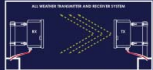
Mounting transmitter and receiver on the edge of a buildings roof top provides a clear path for line of sight and ensures optimum signal strength.
